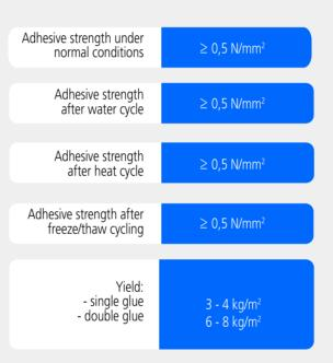
Data based on tests carried out under normal laboratory conditions 23  $\pm$  2°C and 50  $\pm$  5%HR < 0.2 m/s
