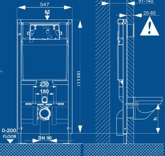
INSTALLATION NOTE: The weight of a wall hung toilet pan can damage or crush the wall lining if plaster board is used. Therefore it is imperative that wall hung pans must only be installed against a non-compressible wall lining such as tiles or other cement based products.
