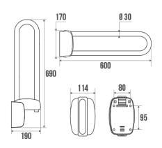
White epoxy-coated aluminium tube Ø 30 mm. Synthetic resin flange. Vertical locking.
