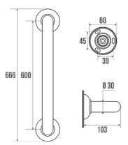
Concealed fixings. White epoxy-coated aluminium tube Ø 30 mm. White resin flanges Ø 65 mm.
